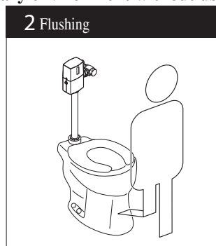
When the user stays in place longer than 10 seconds then moves away, the controller sends a signal to the operating unit to automatically trip the flush valve.
